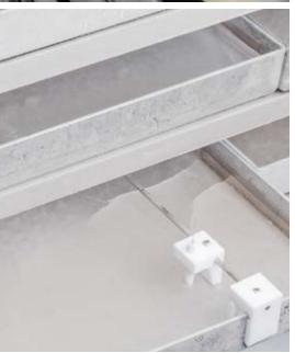
For process optimization and monitoring, the drying speed should be continuously determined in order to ensure safe and economical operation through targeted changes to the process parameters vacuum and shelf temperature. Conclusions about sublimation and the end of the process can be drawn by using PAT tools.
