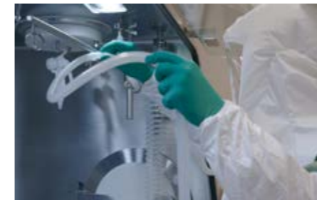
Insertion of single use filling hose
