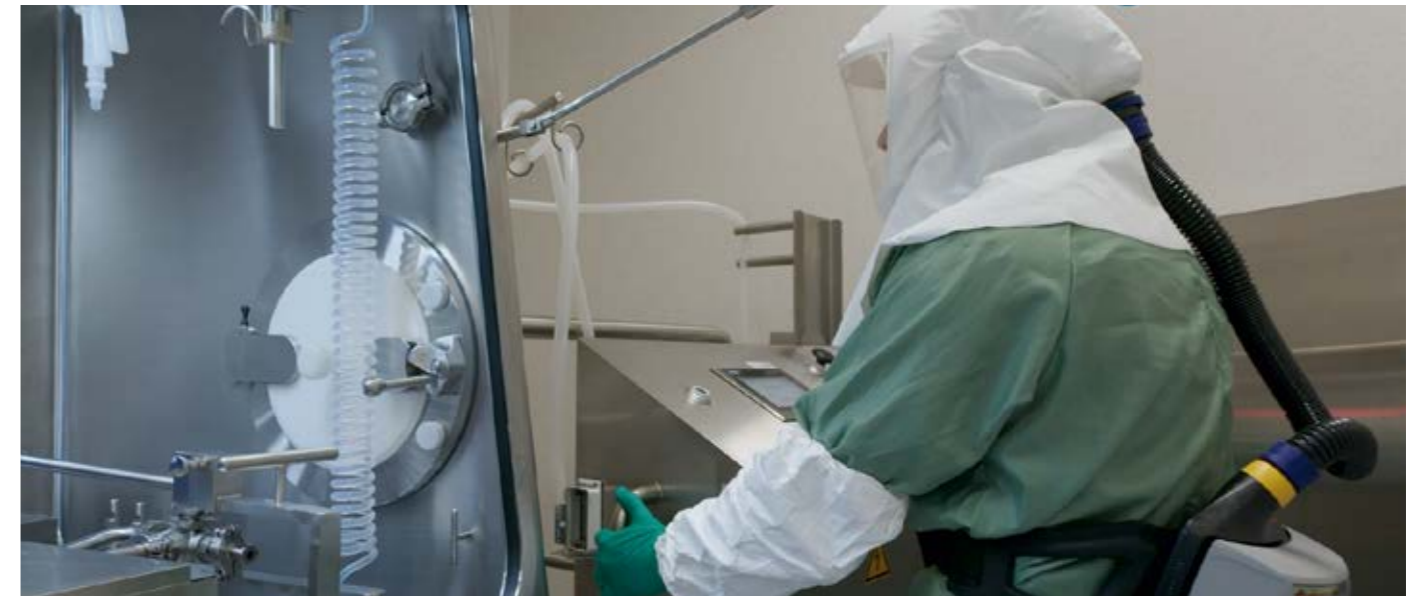
Mobile filling system positioned at isolator
